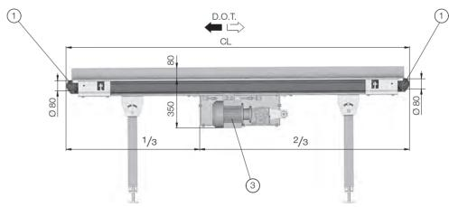
Fig.: Interroll Belt Conveyor BM 4081 (Center Drive)
