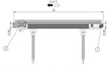
Fig.: Interroll Belt Conveyor BM 4081 (Head Drive)
