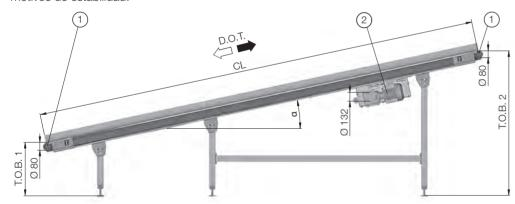
Fig.: Interroll Belt Conveyor BM 4081 Inclined/Declined (Center Drive)
