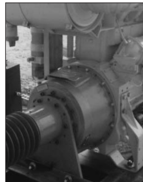
Wichita PTO mounted on Caterpillar diesel engine.
